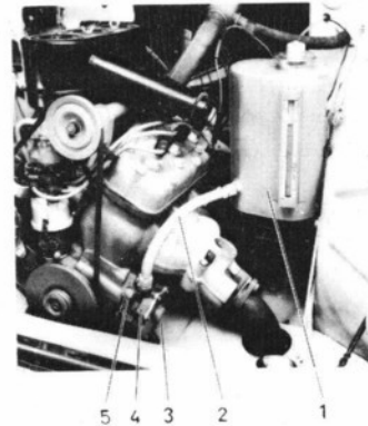
Oil reservoir and pump S 118
